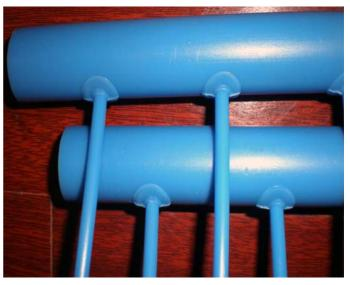
Capillary Tube Mat system is an innovative technology developed to replace the conventional heating and cooling system. Capillary tube is extremely thin pipe made of Polypropylene, carrying water throughout the piping system to exchange heat with the space air by radiation. Capillary tube can be installed on roof, wall, and floor, under the surface decorative materials.
