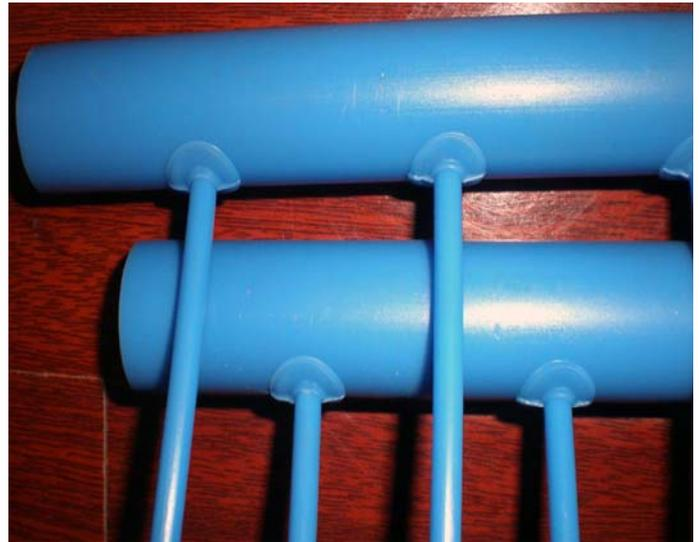
Capillary Tube Mat system is an innovative technology developed to replace the conventional heating and cooling system. Capillary tube is extremely thin pipe made of Polypropylene, carrying water throughout the piping system to exchange heat with the space air by radiation. Capillary tube can be installed on roof, wall, and floor, under the surface decorative materials.
